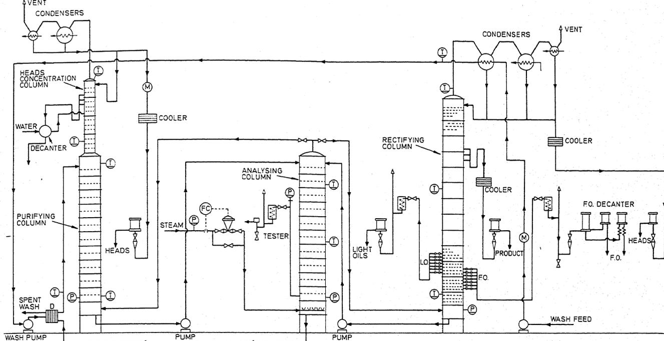
Fig. 2. Flow diagram of a typical rum distillation plant
